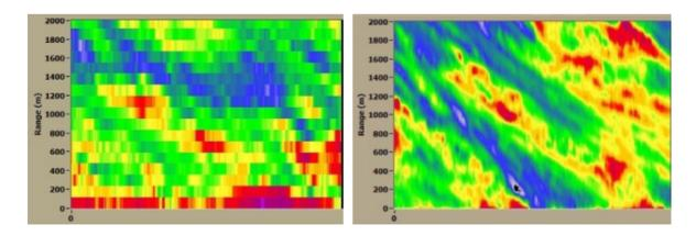
The above data examples show the advantage of utilising a powerful real-time signal processing system. The left plot shows regular acquisition mode with 120m gate length and 2km range = 17 gates. The right plot shows the same 2km range and the same 120m gate length, but now each gate is moved forward by 1.5m instead of 120m, so there are now 1333 gates making up the very much more detailed plot.
