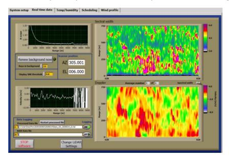
This screen shot shows the XR+ collecting high resolution data. The bottom colour plot shows radial velocity versus range out to 750m. The upper colour plot shows the corresponding spectral width.
